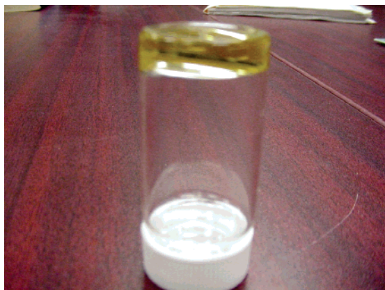
Figure 3. Gel formed from PVP and bimetallic compound 3b (5% functional group equivalents) at 100 mg/mL in DMSO.
